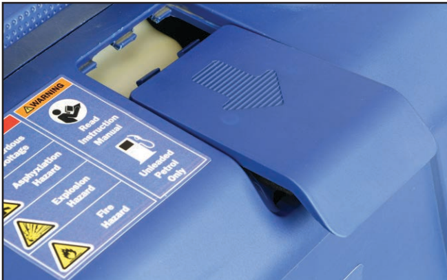
Figure 24 – Removing the Spark Plug Access Cover
