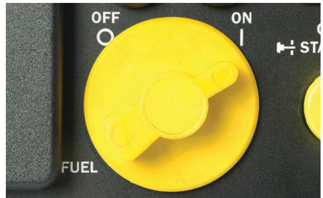
Figure 8 – Fuel Control Switch in the ON Position
