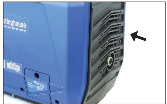
Figure 31 – Cooling Air Outlet Ports
