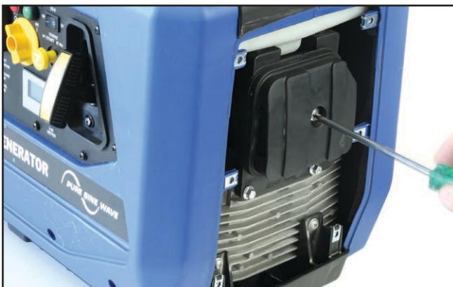
Figure 20 – Removing the Air Filter Cover
