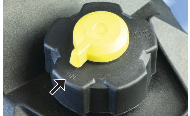
Figure 7 – Fuel Cap Vent in the ON Position
