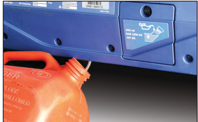
Figure 34 – Collecting Drained Fuel
