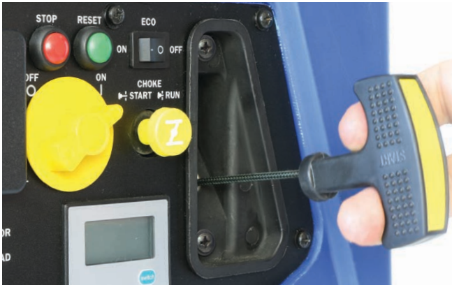
Figure 10 – Recoil Starter Handle Operation
