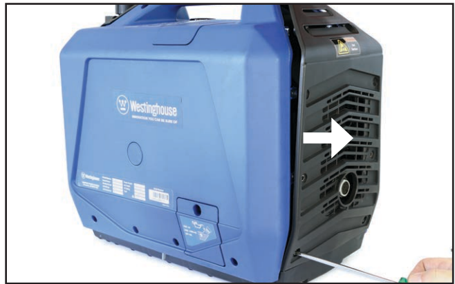
Figure 28 – Removing the Muffler Access Cover
