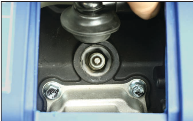
Figure 25 – Removing the Spark Plug Boot
