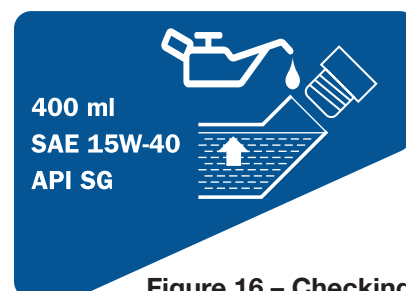
Figure 16 – Checking Oil Level
