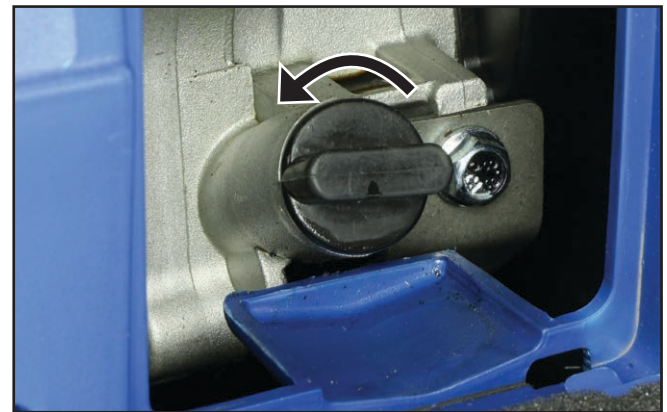
Figure 15 – Removing the Oil Fill Plug
